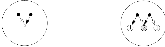
Figure 14.1: In the vector voting scheme, a vector from each landmark (solid circle) to the goal (small triangle) is learned during training trials (left). In later probe trials (right), these vectors are applied to all the perceived landmarks. The location with the most votes is searched. From Touretzky and Redish (1996).
