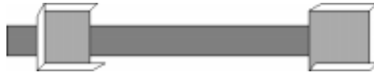
Figure 2.19: The linear track used by Gothard et al. (1996a). Two boxes sit on a linear track. The left box can be moved to any position along the track, varying the effective length of the track.
