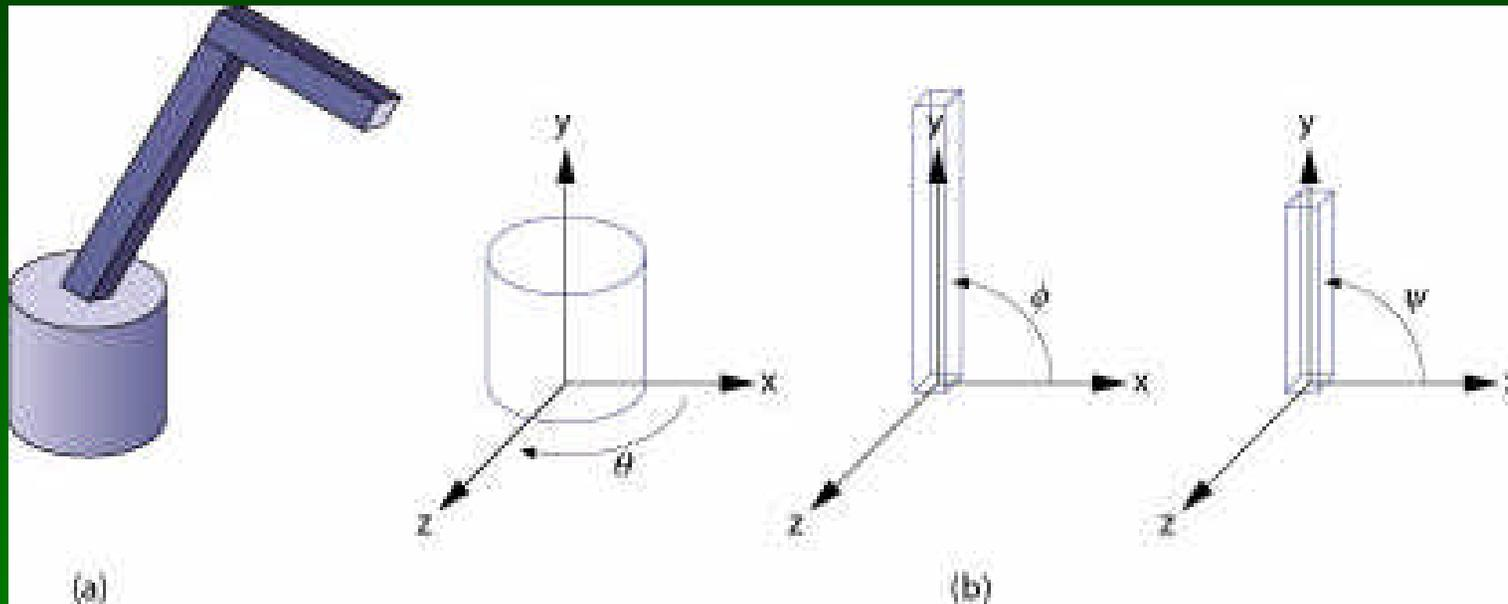
Base rotation  $\theta$ , arm angle  $\phi$ , joint angle  $\psi$
