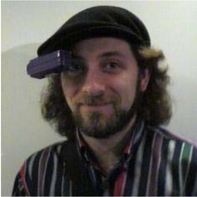
Figure 1. Personal memory aids can help people remember where commonly misplaced items are or interrupted tasks. This picture shows a wearable computer that also acts as a memory aid.
