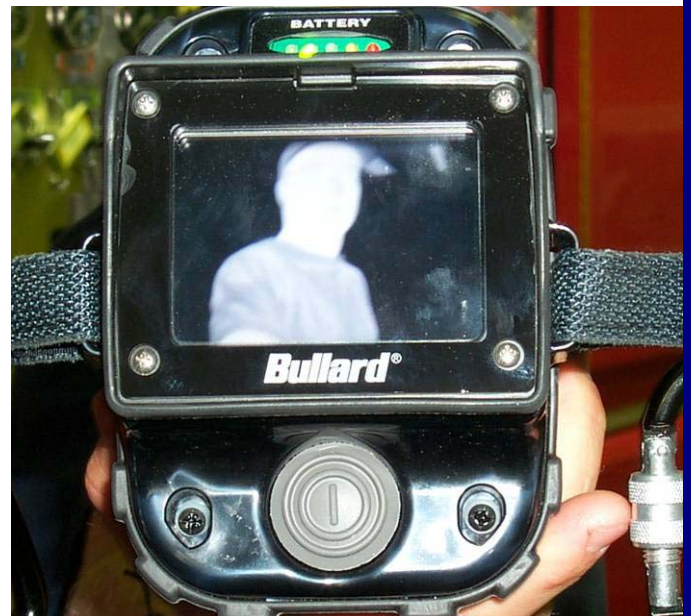
Figure 2. Thermal imagers help firefighters see in the dark and through smoke.
