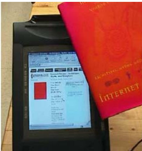
Figure 4. A tag in this book brings a web page in Amazon. One could imagine bringing up reviews for products in stores, such as CDs, books, electronics, and so on.
