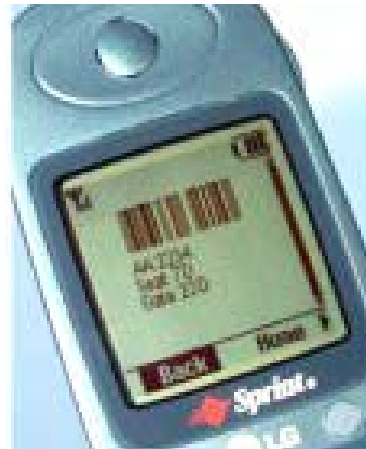
Figure 5. FreedomPass is a security system that uses barcode scanning and voiceprint verification for check-ins on planes. Other companies are looking at using barcodes on phones as replacements for tickets to movies and baseball games. People can purchase tickets using their phone and then use their phone as the ticket.
