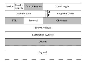
Fig. 1. The fields of an IP packet. Fields in gray are masked out before digesting, including the Type of Service, Time to Live (TTL), IP checksum, and IP options fields.
