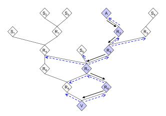
Fig. 6. Reverse path flooding, starting at the victim's router, V, and proceeding backwards toward the attacker, A. Solid arrows represent the attack path; dashed arrows are SPIE queries. Queries are dropped by routers that did not forward the packet in question.
