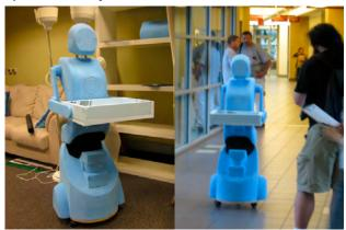
Figure 5. Full-scale mock-up of the robot.
