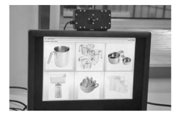
**FIGURE 6.5** A small eye contact sensor was mounted on top of the monitor where the cooking tools are displayed to detect whether the participant is looking in the direction of the monitor. (From Torrey et al., 2007.)
