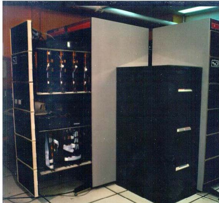
Figure 3. Two of the five clusters of Cm*. The open cluster has four computer modules on the top backplane; K.map is on the bottom.
