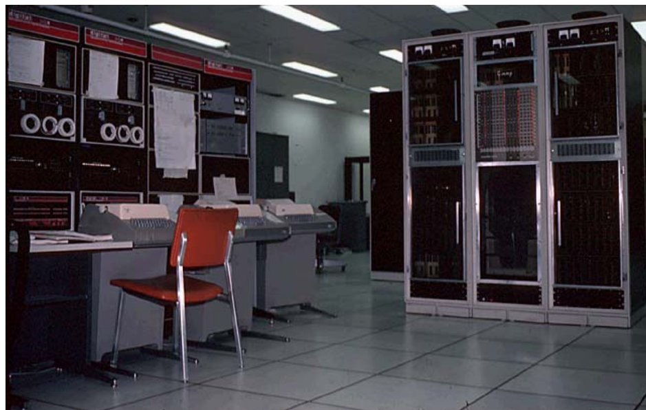
Figure 2. The "H" shaped configuration of C.mmp with crossbar switch and memory in the center, surrounded by banks of four processors.
