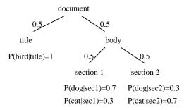
In this diagram, we specified the linear interpolation parameters on the edges. To keep things simple, we use equal parameters for the interpolation. We also specified the language models for the leaf nodes. It is simpler to support unstructured queries, so we will describe retrieval for them first.
