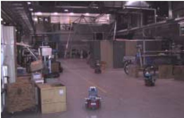
Figure 1: The mapping application was implemented using a team of Pioneer robots equipped with laser rangefinders. The scene depicts the area mapped during the experiments. Note that the environment is very cluttered.
