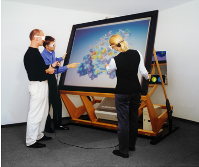
Figure 19.3: A single-screen 3D projection system.
