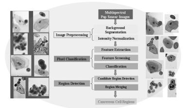
A hierarchical structure for multispectral Pap smear image screening. Input (left): multispectral Pap smear images, Output (right): Pap smear images with labeled cancerous regions
