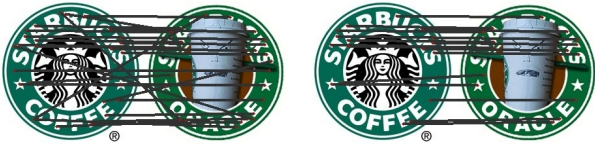
Figure 5: The gray lines represent matched feature points. Matches on the left are the results of individual feature matches. Matches on the right contain the remaining matches after common object verification.
